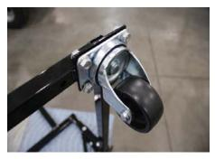
Install casters and tighten bolts/nuts. (1/2" wrench)
