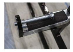
Carraige bolts install through each of the threaded tabs. You may need a 3/8" wrench to help install the carraige bolt through the tab. Thread on Nut and Tigtening Knob. Tighten the nut to the knob using a 1/2" wrench.
