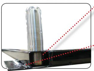
Pins screw in. If you wish, use pliers to snug the pinshowever <u>be certain</u> to use a rag or piece of material as cover to prevent marking/scoring the pins. Thread locker can also be used on the threads to help reduce the chance of the pins loosening during transport.
