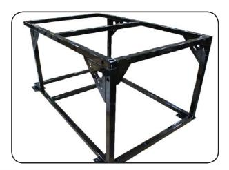
The bottom frame (base) is a full welded piece. The only items needing to be installed are the location pins and the casters. The pins will screw right into each corner of the frame. Hardware for caster installation was included in the caster kit which was shipped in their own box separately from Stacker frame components.
