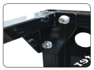
The cross bar with welded gusset tabs will match up and connect to both the horizontal and vertical posts of the upright. At this point you want to be certain to take care while tightening the bolts into weld nuts. These need to be gently tigtened, not cranked on.
