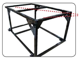
The cross supports get bolted to the main rails. Match the two end supports to their proper bolting location.
