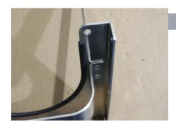
Rivet second Face Plate to Main Bracket.
