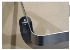
Rivet 1 side plate and Face Plate to a Main Bracket.
