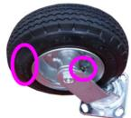
2) Adjust air pressure to specified pressure listed on sidewal
