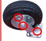
3) Grease/spray-lube spindle, hub and caster swivel plate (if applicable)
