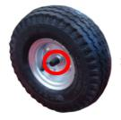
3) Grease/spray-lube hub bearing (if applicable)
